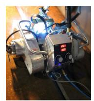
welding process by offloading repetitive control tasks and allowing the operator to focus on bead setup and quality monitoring.
