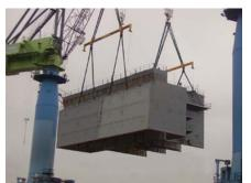
measures remain. The analysis will be verified by using strain gauges on lifts of complex blocks. Additionally, the project will evaluate the use of integrated lifting lugs in place of temporary pad-eyes.
